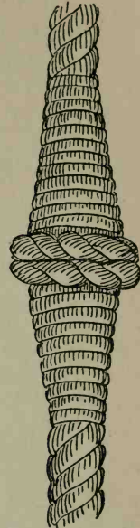
FIG. 120.—French shroud knot (complete).
